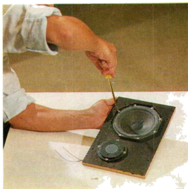
The tweeter has been fitted after staining the baffle black. The woofer is then screwed into position. Washers are placed under the screw heads.
