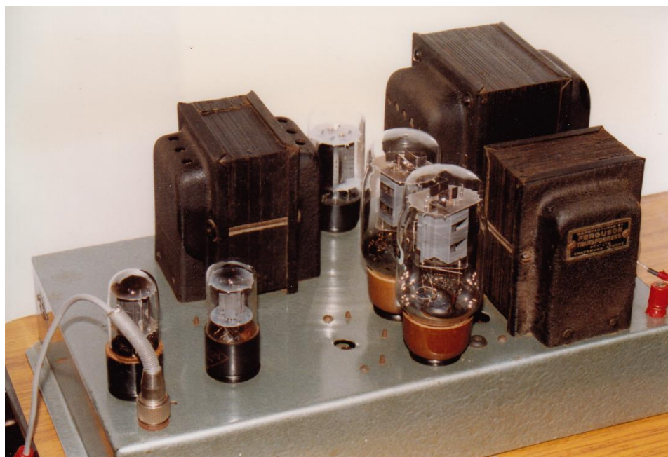
1950. A Williamson amplifier in the slightly revised British format. Marketed by Audio Engineers Pty Ltd Sydney.
