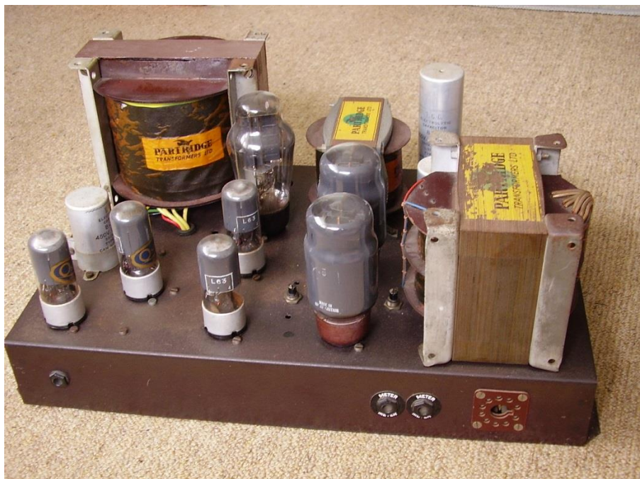
1948. A superbly constructed Williamson amplifier of the early format using four type 6J5 valves for the input stages, made by Rogers Developments, England.
