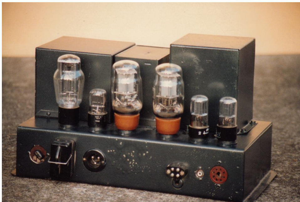
1950. A Williamson amplifier marketed by Goodsell, England. This variant incorporates an auxiliary rectifier 6X5 valve (2 nd from left) for powering attached pre-amps etc.
