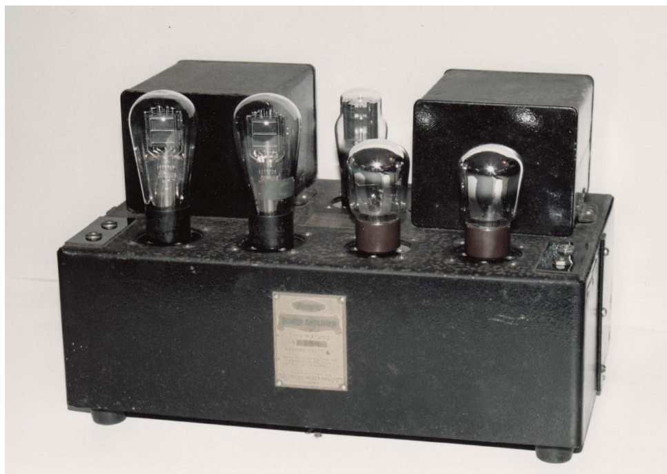
1930. A robustly built early audio amplifier by EMMCO, Australia. Push pull triode output with interstage transformer drive. The output is at high impedance requiring a loudspeaker with its own transformer. 4-5 watts.
