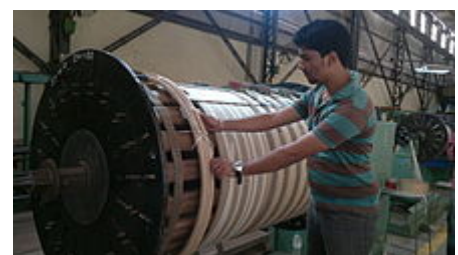
Winder checking insulation at lathe.
